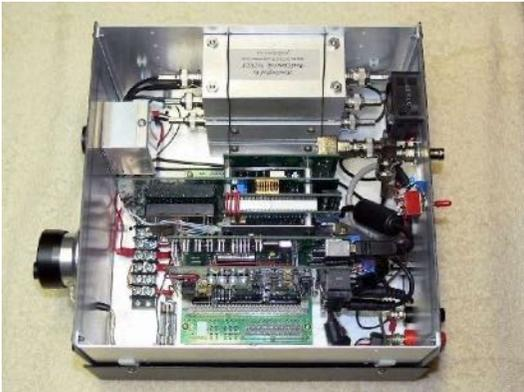
FlexRadio SDR-1000 receiver combined with custom-made high-pass and low-pass filters, integral sound card, and tuning knob, circa 2007.
