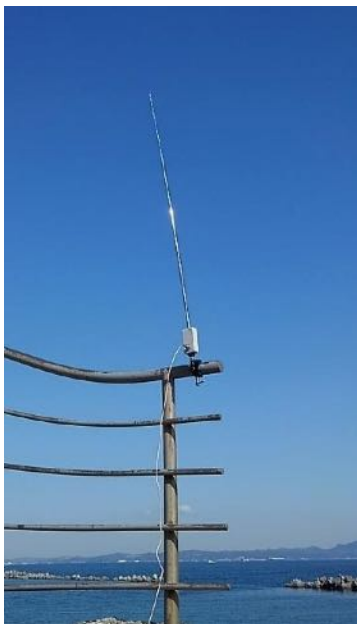
Active Whip Antennaを手摺りに取り付け
