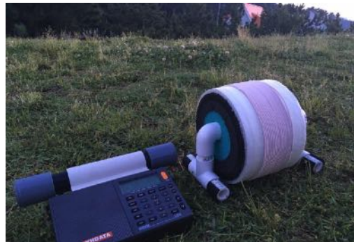
Modified D-808 with new ferrite, and 5’ Frequent Traveler’s FSL by Gary DeBock san.
