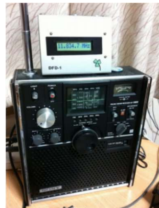
My Skysensor ICF-5800 that I am still using even now. There are a few minor damages and replacement, but still works fine. A frequency counter is added for direct reading.
